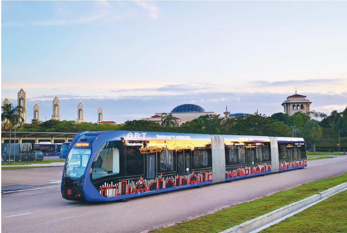
The ART carriages run on rubber wheels and, with the use of optical sensors, follow a virtual track painted on the road using regular road-marking paint (Photo by Mobilus)
